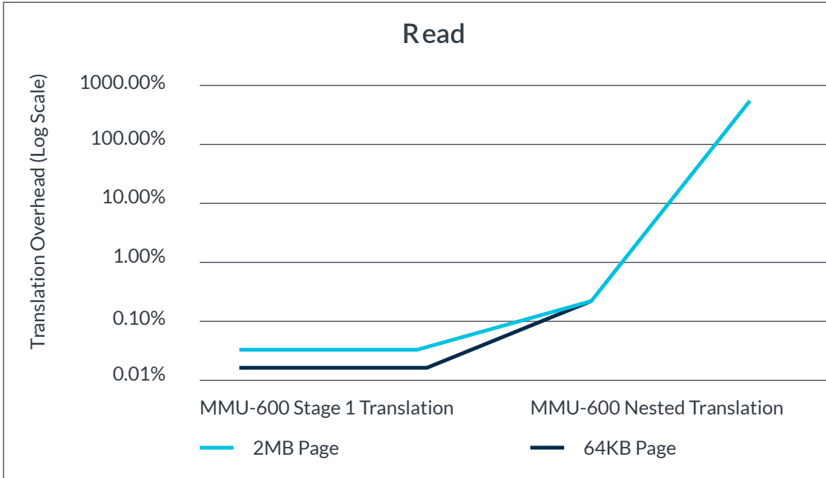
Figure 3: MMU-600 read translation overhead compared to Software (lower is better)
