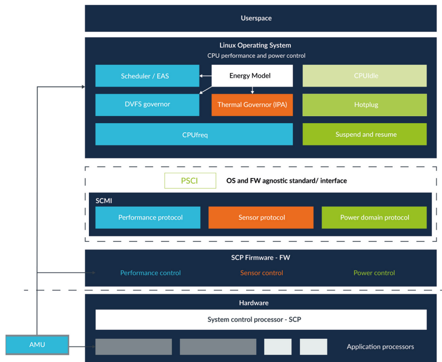
Figure 2: Linux power and performance management architecture and SCMI
