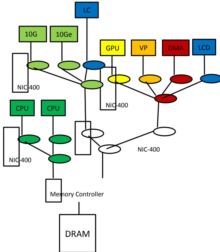
Each switch can select the appropriate data width and clock frequency to meet performance target while minimizing power and area. Different switches can be placed in different domains allowing hierarchical clock gating to reduce power whenever each domain is idle.
