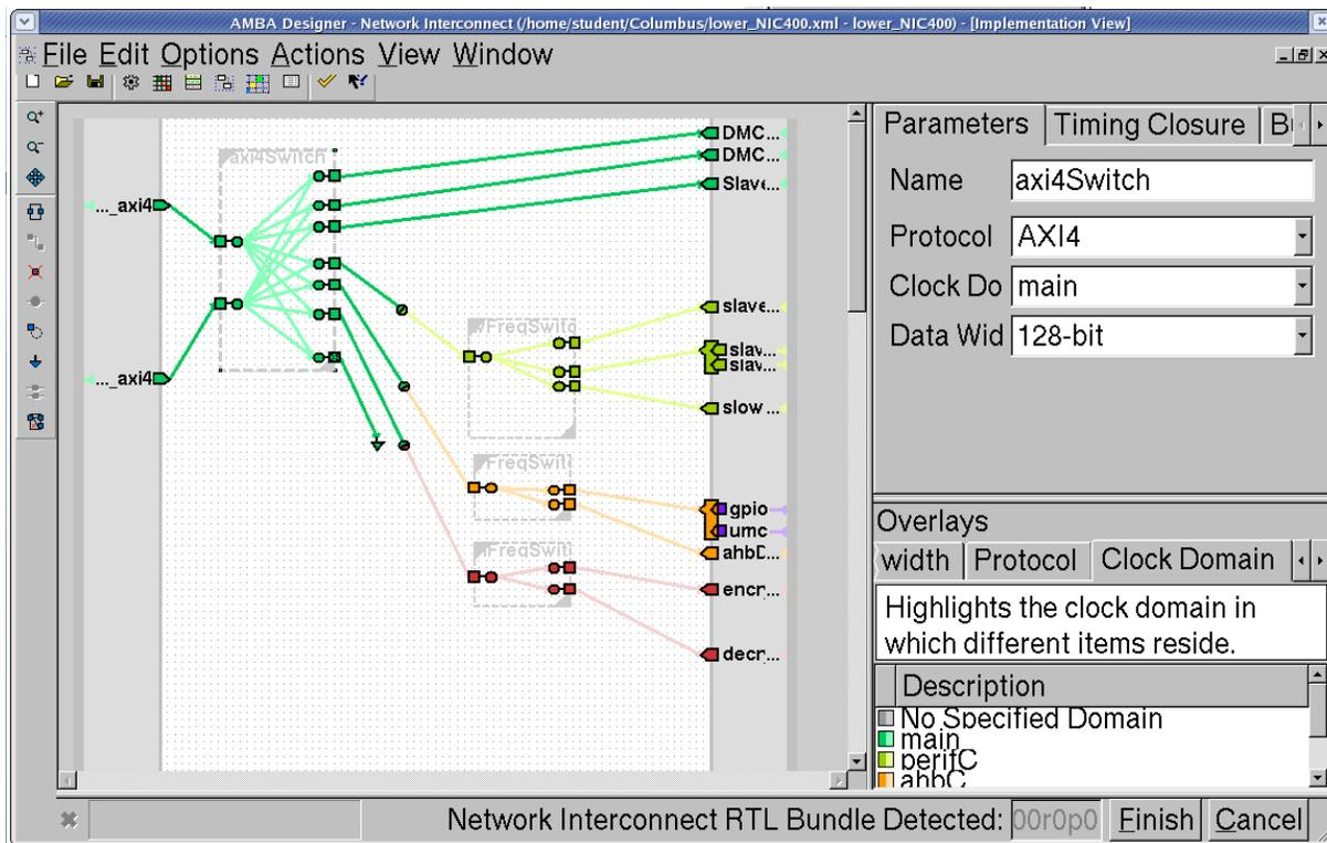
The designer can add Thin Link bridges to bridge between remote masters and slaves and NIC-400 instantiations with fully configurable wire count, bandwidths and latencies.
