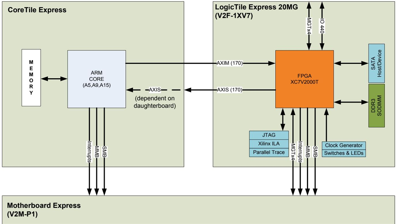
The upper connectors allow the user to develop their own breakout board for connection to Si e.g. modems or to connectors to other systems or interfaces. It is possible to add an additional LTE 20MG on top for additional FPGA prototyping space.
