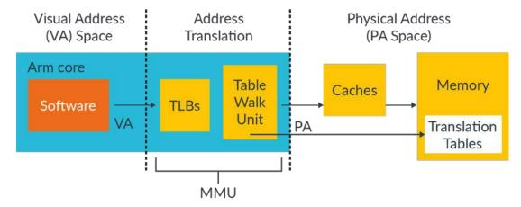
A virtual address must be translated to a physical address before a memory access can take place (because we must know which physical memory location we are accessing). This need for translation also applies to cached data, because on Armv6 and later processors, the data caches store data using the physical address (addresses that are physically tagged). Therefore, the address must be translated before a cache lookup can complete.
