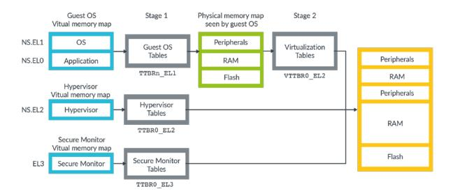
The diagram shows three virtual address spaces:
