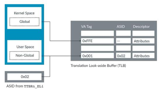
The diagram shows that TLB entries for multiple applications are allowed to coexist in the cache, and the ASID determines which entry to use.
