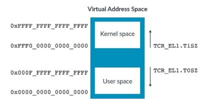
The virtual address size is encoded as:
