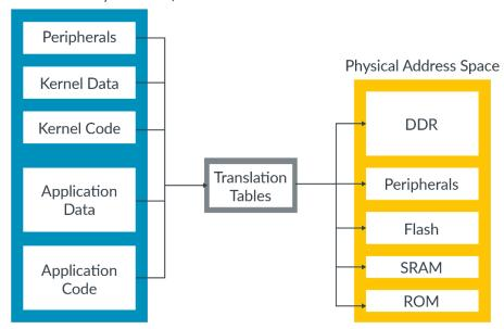
Translation tables are in memory and are managed by software, typically an OS or hypervisor. The translations tables are not static, and the tables can be updated as the needs of software change. This changes the mapping between virtual and physical addresses.
