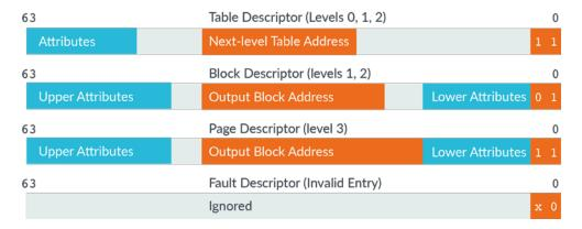
Note: For purposes of clarity, this diagram does not specify the width of bit fields. You can find this information in the Arm Architecture Reference Manual Armv8, for Armv8-A architecture profile: The VMSAv8-64 translation table format descriptors.
