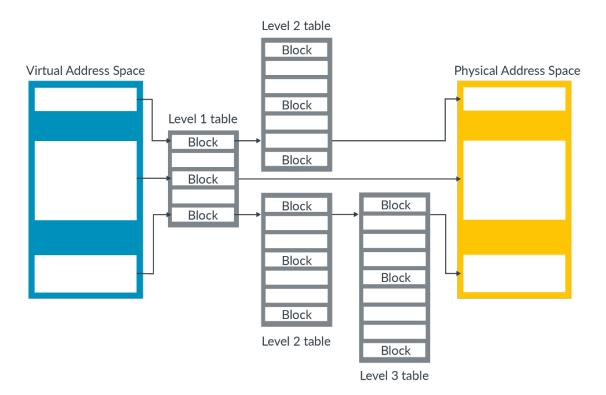
In Armv8-A, the maximum number of levels is four, and the levels are numbered 0 to 3. This multilevel approach allows both larger blocks and smaller blocks to be described. The characteristics of large and small blocks are as follows:
