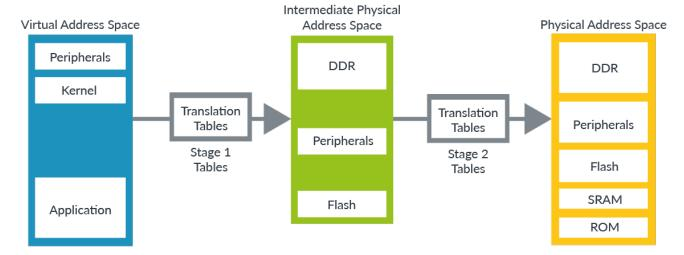
Although there are some minor differences in the table format, the process of Stage 1 and Stage 2 translation is usually the same.
