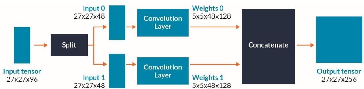
The grouping convolution not only allows you to spread the workload over multiple GPUs, it also reduces the number of MACs needed for the layer by half.
