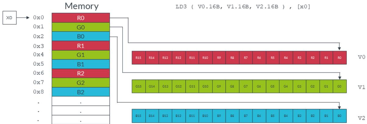
The red and blue values can now be switched easily using the `MOV` instruction to copy the entire vector. Finally, we write the data back to memory, with reinterleaving, using the `ST3` store instruction.
