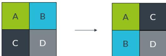
We can use the Neon transpose instructions to transpose matrices.
