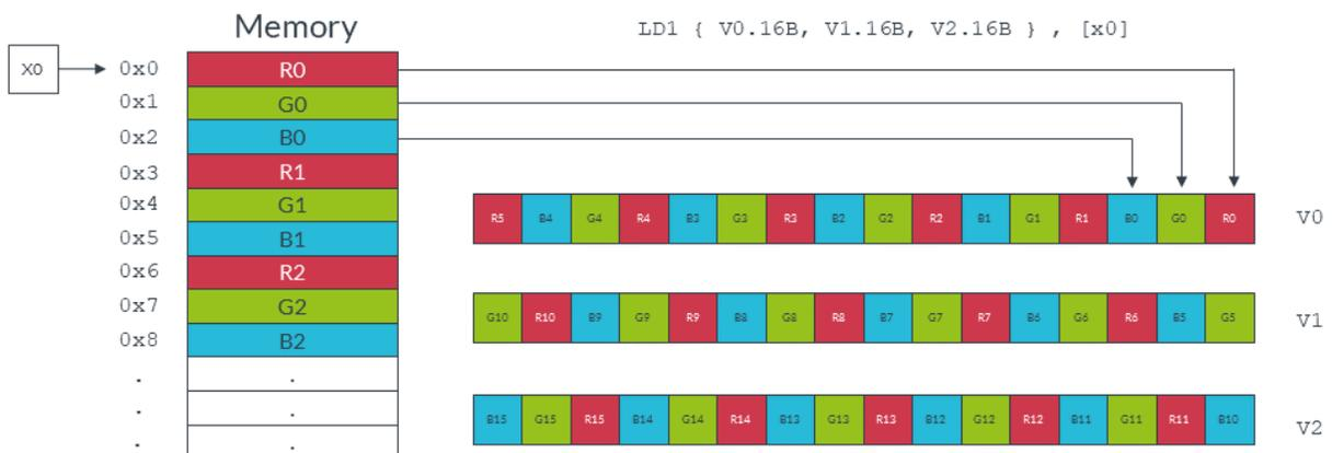
Code to swap channels based on this input would be complicated. We would need to mask different lanes to obtain the different color components, then shift those components and recombine. The resulting code is unlikely to be efficient.
