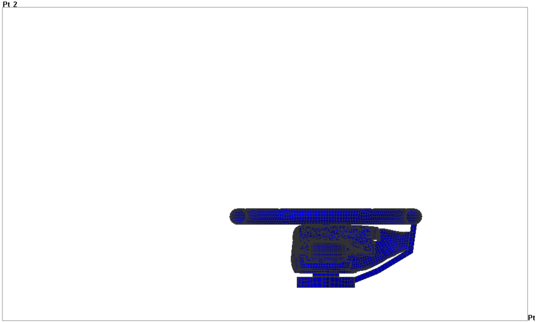
Driver airbag unfolding out of a steering wheel (cut view) FPM velocity vectors
