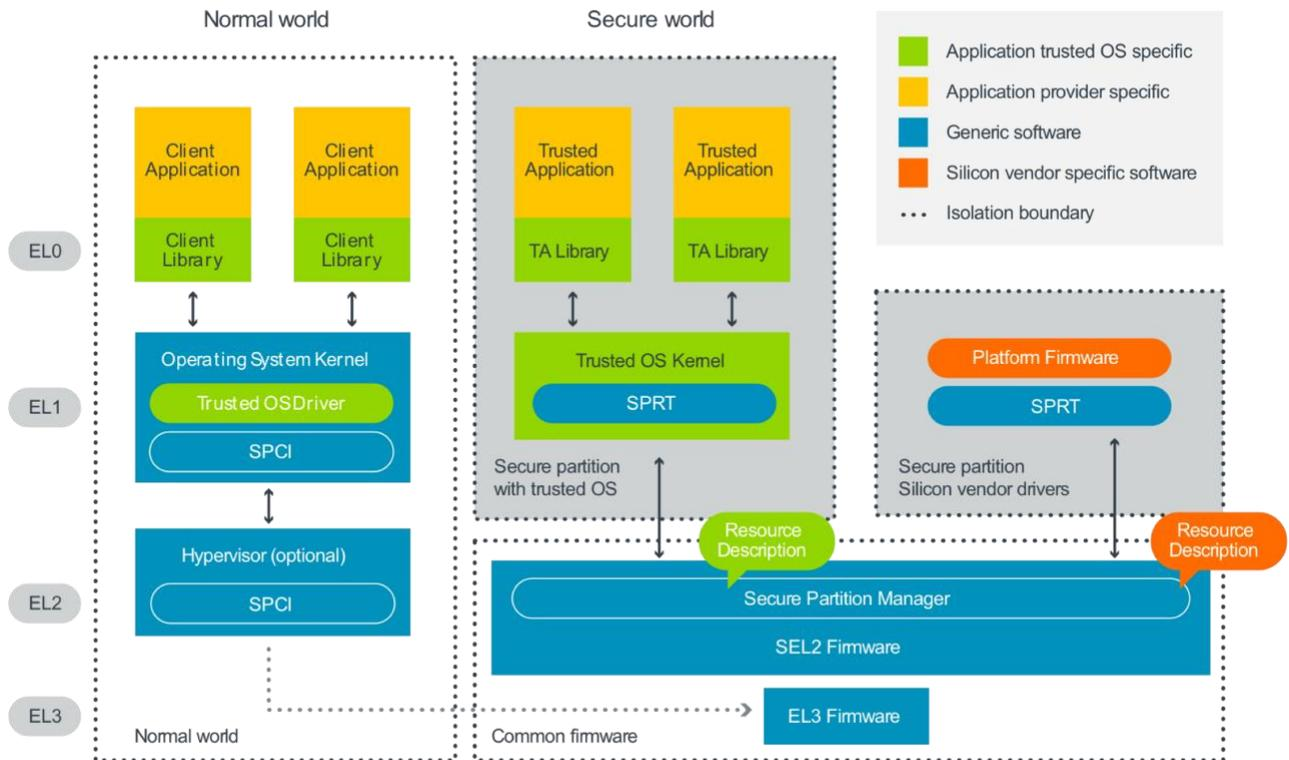
Figure 3 Software stack with secure partitions
