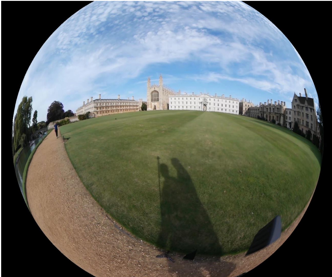
Figure 5: Equirectangular video mapped to a sphere as seen from outside the sphere
